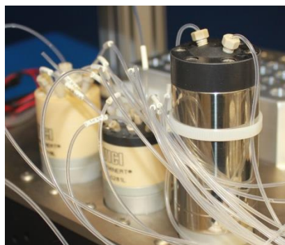
Figure 4: 10-port selection valve (left), 18-port selection valve (center) and milliGAT pump (right)
